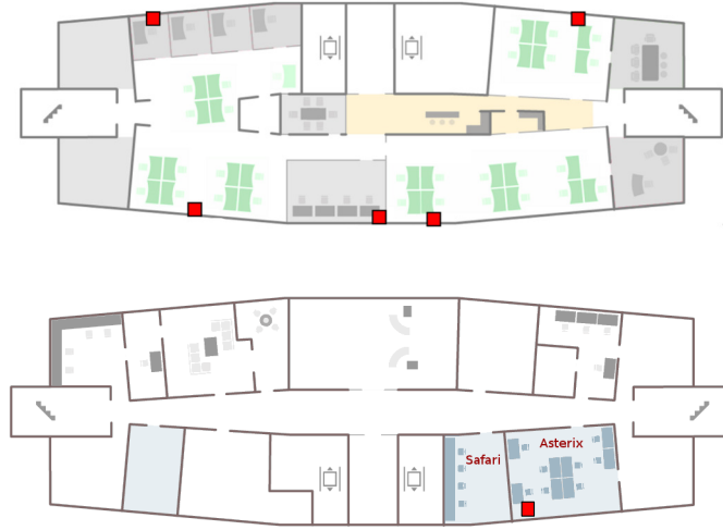
Figure 6.1: The x86 based wireless testbed in an office environment on the 15 th (bottom figure) and 16 th (top figure) floors of the TEL building at TU-Berlin. The red squares indicate the positions of the APs that comprise the indoor testbed.
